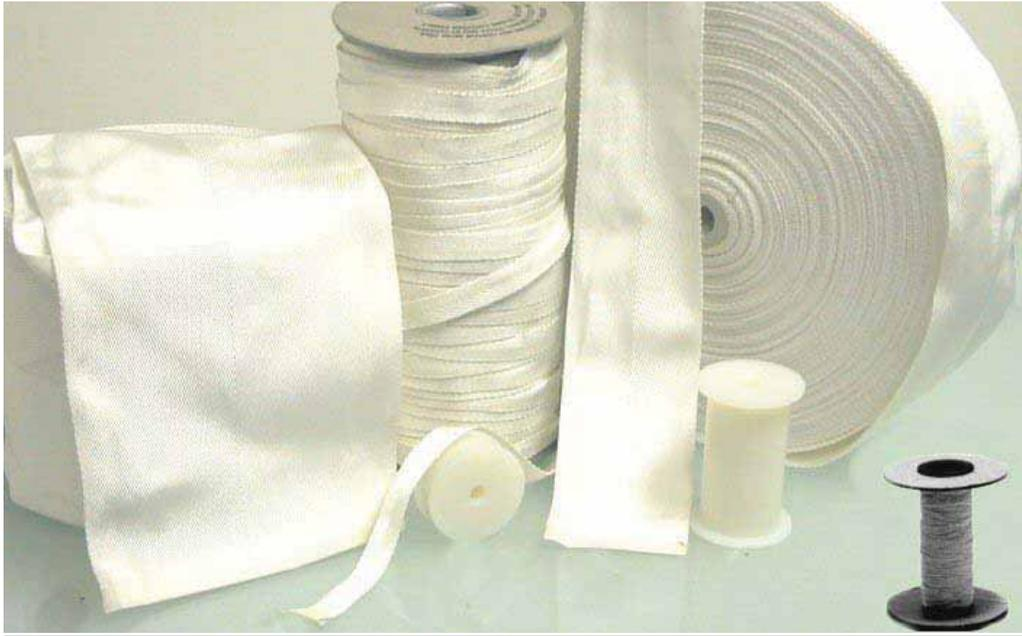
The supplied material is cut to the desired length by the plant and then sewn together with Nomex Thread. Although Epic Nomex material exhibits very low stretch, some stretch will occur over time. If the material becomes slack, cut off excess and re-sew as shown. Most plants sew Nomex belting by hand using a curved upholstery needle or a large straight needle (available from a local sewing notions store) using Nomex thread.
